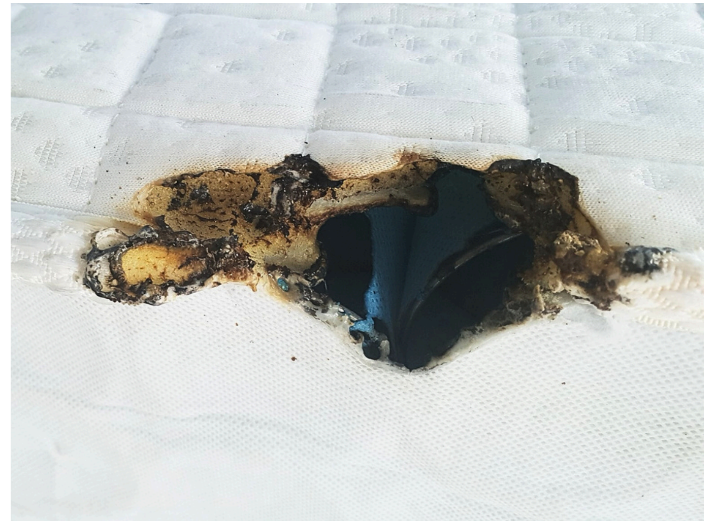
Photo of a match test failure from our Due Diligence Random Testing Programme, which was created to strengthen our Code of Practice.
