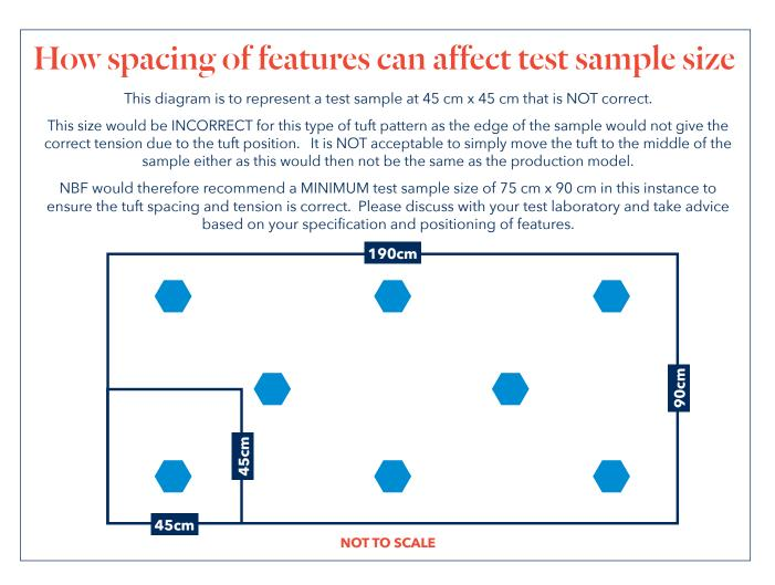
BS 7177 suggests a minimum small-scale test sample size of at least 450mm x 350mm, however in practice many test samples are produced at 450mm x 450mm.
